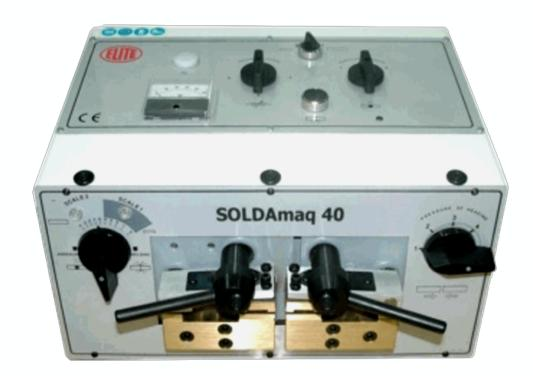
The Elite SOLDAmaq 40 is our bandsaw welding "Push and Go": Just follow the welding parameters we provide you with depending on the thickness and width of the saw, close the saw clamping jaws and push the welding button.
