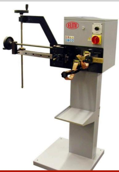
The ELITE SOLDAmaq 1200 is specially designed for its dimensions for sawmill industry but is suitable for every type of carbide tipped circular sawblade.
