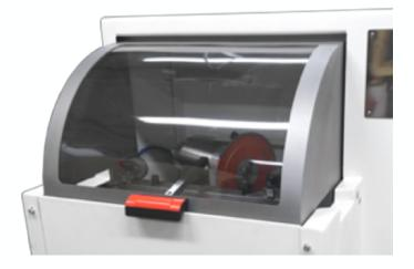
Cabin in stainless steel, to avoid the corrosion produced when sharpening with cooling.
