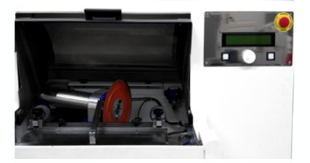
Control panel integrated in the cabin. You can create and edit programs with the top view of the teeth to be sharpened, for easier adjustment.
