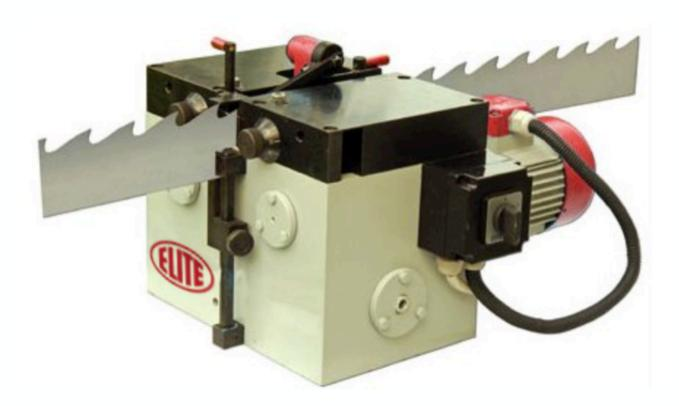
The Elite TR-5 has been designed for the heaviest of setting works, as it can set the teeth on band saws with a width of 20 to 120 mm.
