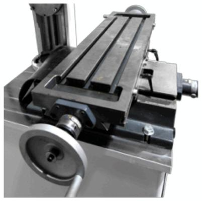
Working table with a load capacity of up to 100 kg movement by means of rectified steel guides with comfortable hand wheels for front and longitudinal movements.
