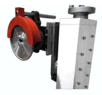
Detail of grinding wheel holder with protection for grinding wheels up to Ø150 mm. The grinding wheel head can be rotated 360° with respect to its vertical axis and 90° with respect to the horizontal axis.
