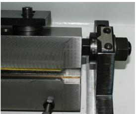
**Image 1**: **1 CV grinding wheel motor.** Displacement of the lowering of the grinding wheel by means of guides with ball recirculation skids. Head mounted on precision linear guides.
