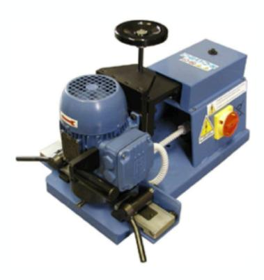
Can be optionally equipped with SOLDAmaq EC deburring machine, for removal of the weld burr
