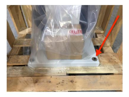
Once the machine is moved to its final working destination, you must fix the machine to the floor by means of the 4 screws placed in the machine base stand.
