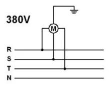
Only the earth cable can be connected with the yellow-green cable in the middle (earthing).
