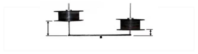
The roll for SETTING must be positioned 3-4 cm. from the horizontal rod. The roll for SHARPE-NING must be positioned 15-20 cm from the horizontal rod.
