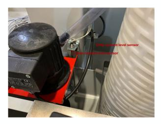
Dirty and clean liquid level sensor to control the status and flow of the coolant and decide if the filter tank should be filled automatically.
