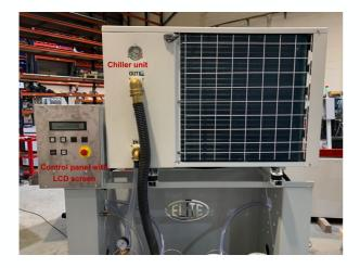
View of the filtration system with the cooling system mounted (Available as an option).
