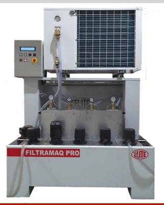
The new ELITE FILTRAmaq PRO, is our autonomous equipment for the filtration and cooling of liquids, up to 2µm. It represents a renewed and improved version of the previous model.
