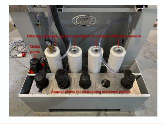
Pumping of the clean liquid by means of the pump of the sharpening/grinding machine itself. Very easy to change filter cartridge system.
