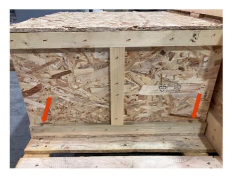
To remove the machine from its packaging, first remove the shears (blue arrow), and then remove the wooden blocking pieces (red arrows).
