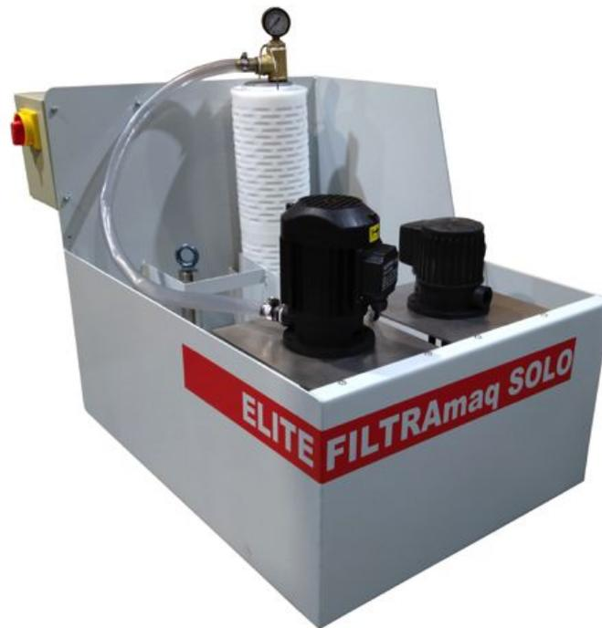
The new ELITE FILTRAmag SOLO, is our autonomous equipment for the filtration of grinding/sharpening liquids, up to 2 $\mu$ m. It represents a renewed and improved version of the previous model.
