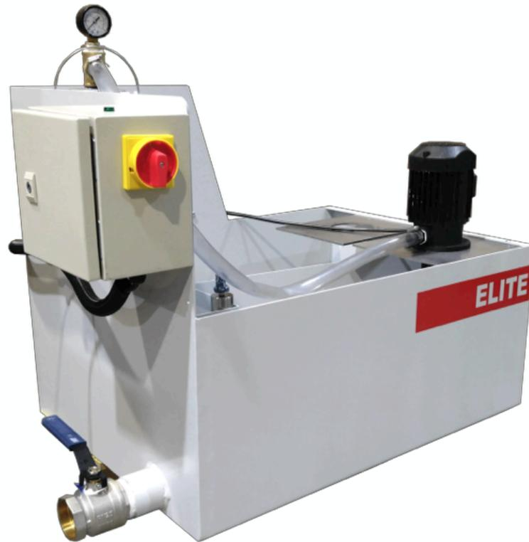
Detail of dirty coolant inlet: via a 2" female connector.
