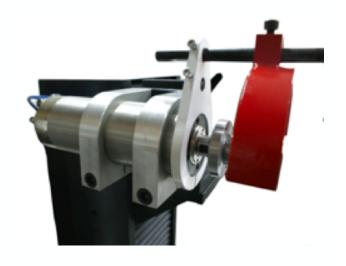
Direct grinding wheel motor for full power (2 HP) with variable speed drive from 3000 to 9000 rpm
