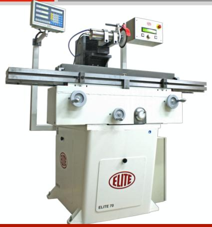
The ELITE 70 is our high precision and robust universal tool and cutter sharpening machine, designed for the toughest jobs, as it allows to load up to 200 kg on the working table, achieving accuracy of microns for the most demanding sharpening or grinding of your cutting tools.
