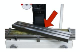
Work table with 360° rotation, to be able to work from all the positions that are required, it has graduation for a precise adjustment of the position.
