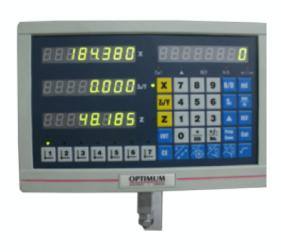
Control panel with digital scale position indicator. Up to 3 axis: X, Y, Z available as an option.
